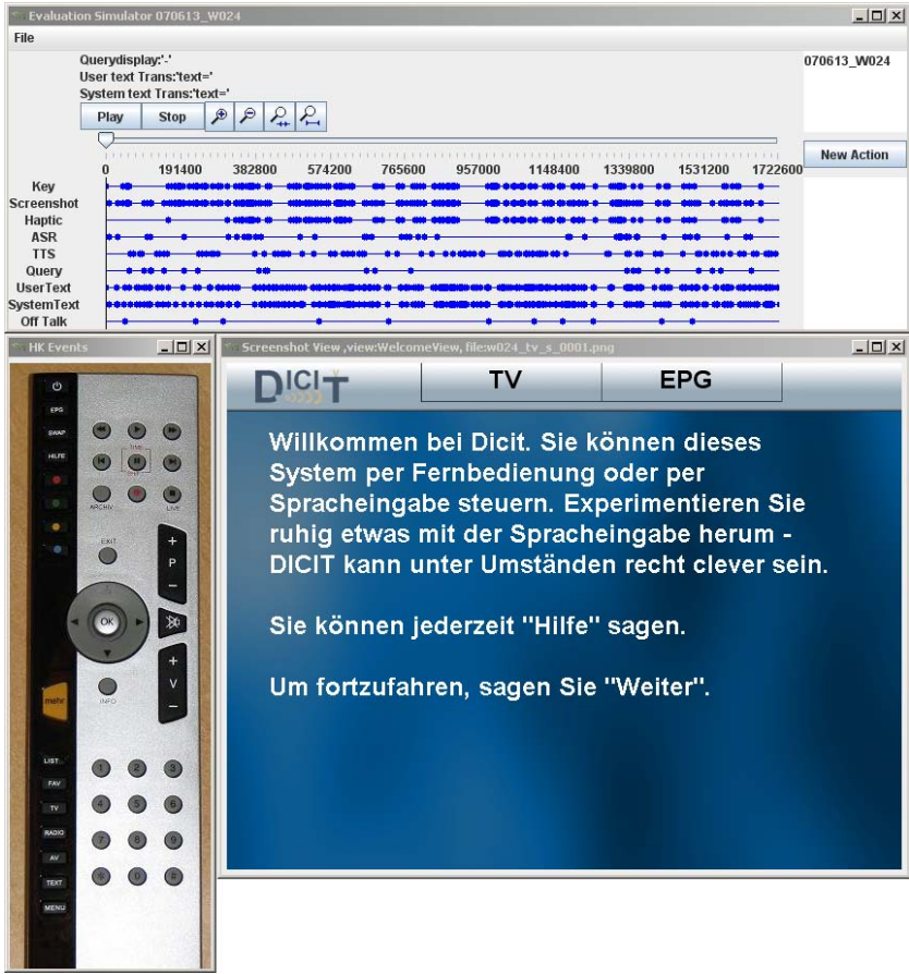
Fig. 1. The main windows of the evaluation tool showing the the DICIT log data, including a screenshot of the current view and a remote control visualization
