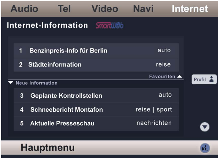
Fig. 1. The SmartWeb driver interface: buttons are structured into two areas “Favorite items” and “New information”; Labels are assigned to each headline; a profile button on the right activates a personalization screen
