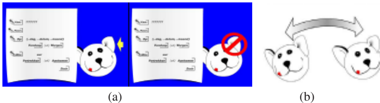
Fig. 3. Visualizations for Iteration 3: (a) HCI concept. Left panel: utterance intended for system. Right panel: utterance intended for partner. (b) CA concept – rotating bear face: when the utterance is assumed to be intended for the system, the face is turned towards the speaker; when the utterance is assumed to be intended for the partner, the face is also turned towards the partner.
